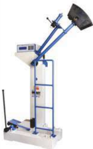
Impact Testing Machine
